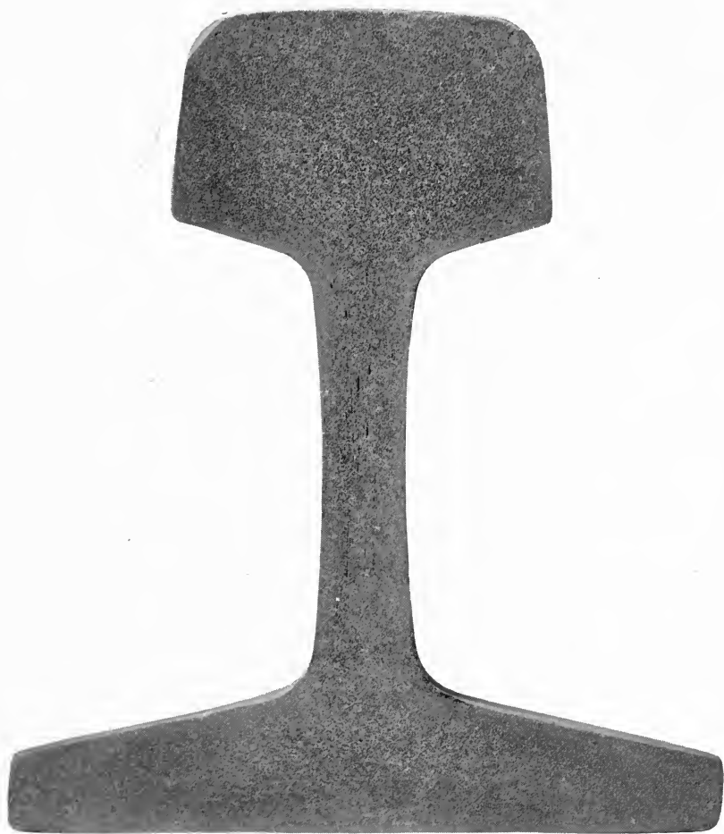
VANADIUM STEEL HEAT 26813, RAIL "B" Shows a very solid, uniform, dense structure.
